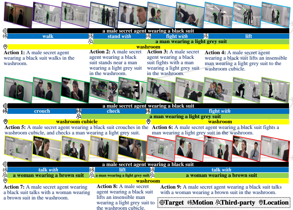
Figure 4: An example of action annotation. We label the target, motion pattern, third-party object, and scene for each action . The target to be tracked is determined in the first frame and does not change during the entire video sequence. A change in any of the other three elements will end the current action and proceed into the following action .
