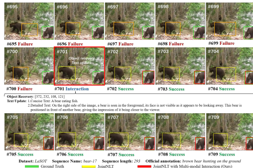
Figure 1: Example of tracking with multi-round multi-modal interaction. We provide the tracker with the correct bbox and a more accurately aligned concise/detailed text through interaction.
